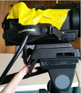
Plug the micro-HDMI end of the HDMI/microHDMI cable into the camera, connect the regular HDMI plug with the Galicaster's HDMI input. Connect the camera's power cable and plug it into a power outlet.
